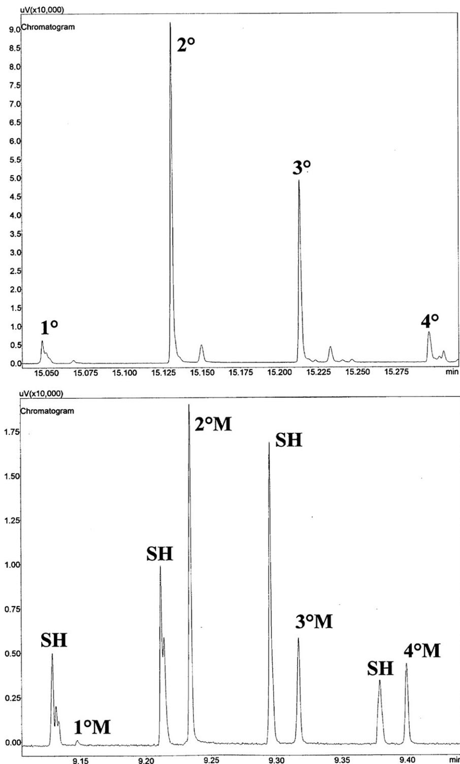
**Fig. 5.** Untransformed chromatogram expansions, relative to the diesel application; 1°, 2°, 3° and 4° refer to the modulation number. Abbreviations: SH, saturated hydrocarbon; MH, monoaromatic hydrocarbon.
