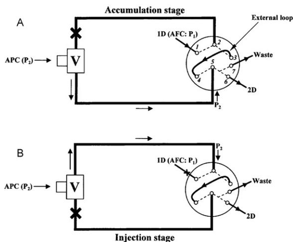
**Fig. 2.** Scheme of the FM accumulation (A) and injection modes (B). Abbreviations: V: 2-way solenoid valve; AFC: advanced flow controller.
