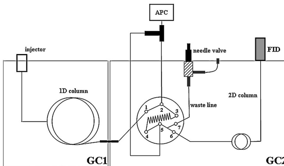
Fig. 1. Scheme of the FM GC  $\times$  GC set-up.
